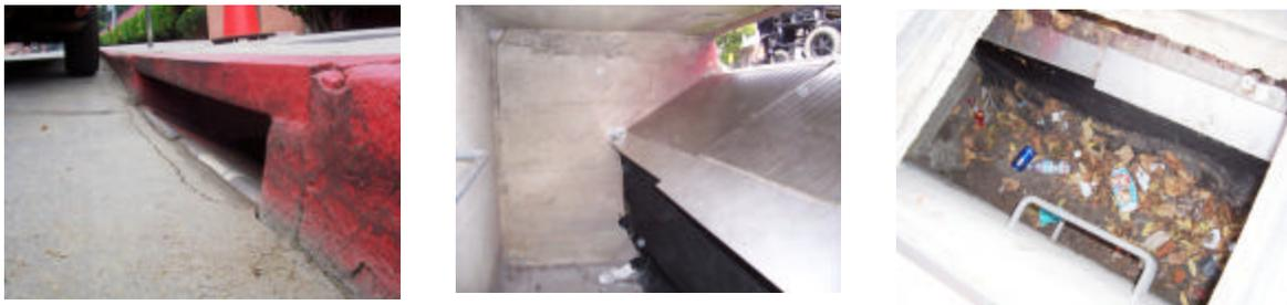
Debris removal efficiency was virtually 100%. The captured debris air-dried quickly and remained in a state of dryness. Sieve analysis of the sediment and grass seeds is shown in the following figure. USC collected water quality samples in the curb inlet and discharge, reporting removal efficiencies of various dissolved constituents shown in the table below.
